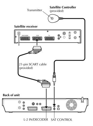
The following procedure is required if you receive satellite channels through a satellite receiver. Approximately 20 seconds before the SHOWVIEW timer programming ( pp. 54) or Manual Timer programming pp. 56) starts, the unit sets its input mode to "L-2" and automatically switches the satellite receiver's channels using a provided Satellite Controller.
